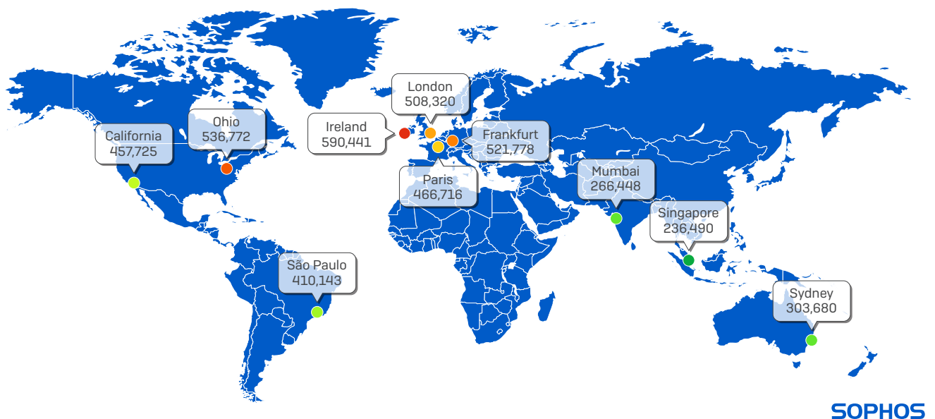
Fig.7. We distributed honeypots to datacenters around the world and permitted attackers to try to brute-force their way in. The honeypot machines were discovered “organically,” without being advertised in any way. Over the 1-month period of our tests, this map illustrates how many attacks each honeypot location received.
